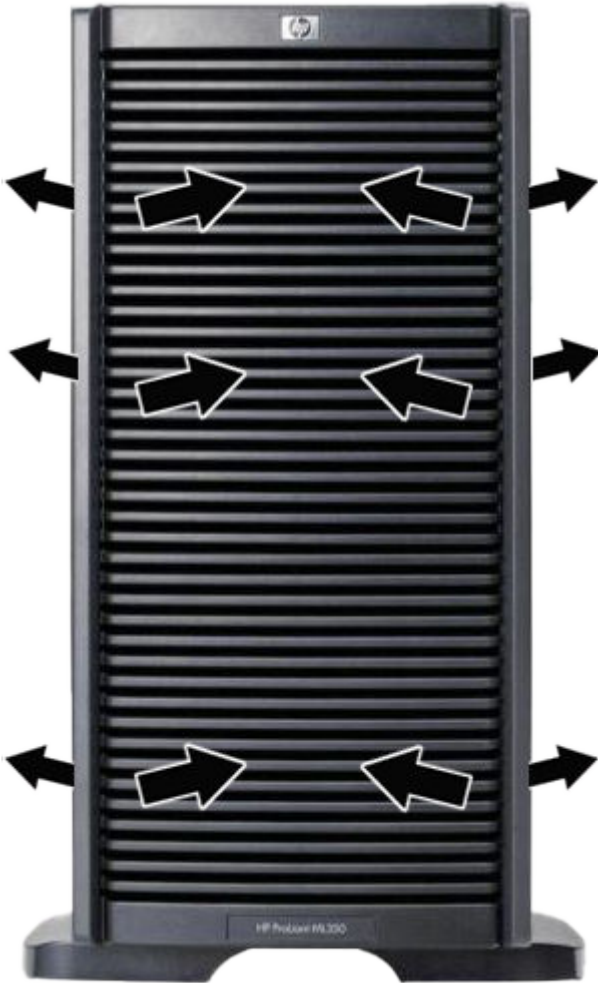
Figure A-17 Air flow of the HP ProLiant ML350 G6 Server
